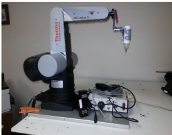
Fig. 1 - Robotic arm of the typical CRS robot system 3
