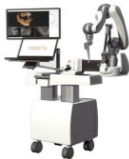
Fig. 3 - Yomi dental implantology robotic system 3
