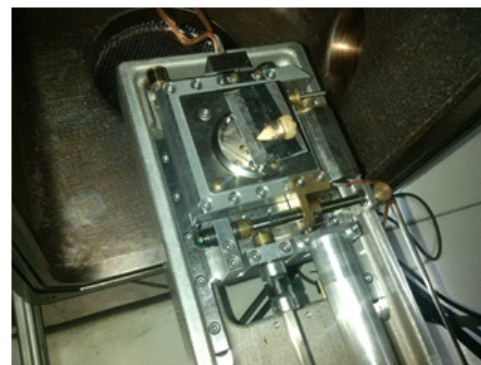
PHOTOGRAPH 4: Mounting of the specimen before sealing the vacuum chamber
