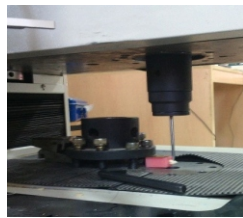
Figure 5: Force application on the lingual side of sample
